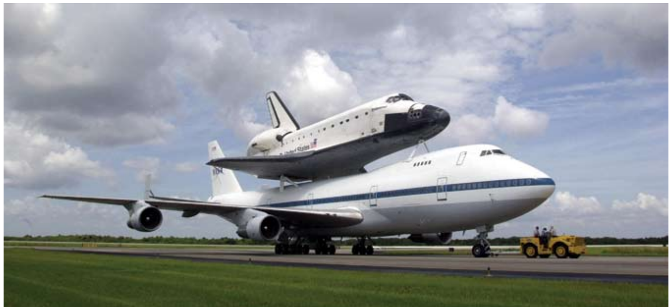
Space Shuttle Endeavour is towed toward the Mate-Demate Device following landing on runway 15 at KSC's Shuttle Landing Facility atop a modified Boeing 747 Shuttle Carrier Aircraft.
