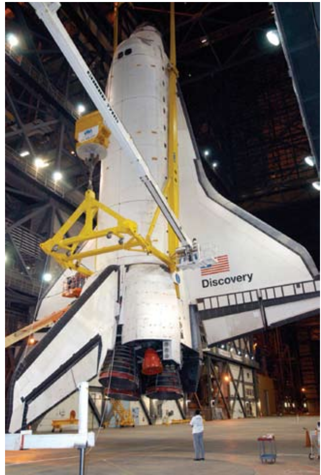
A 175-ton bridge crane in the Vehicle Assembly Building lifts Discovery to move it into High Bay 3 for mating with the External Tank and Solid Rocket Boosters.
