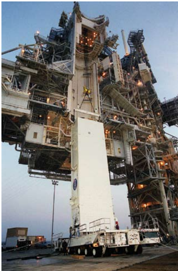
The Payload Canister Transporter can transport payloads in the Canister either vertically or horizontally. On the launch pad (above), the Canister is ready to be lifted up into the Payload Changeout Room on the Rotating Service Structure.
