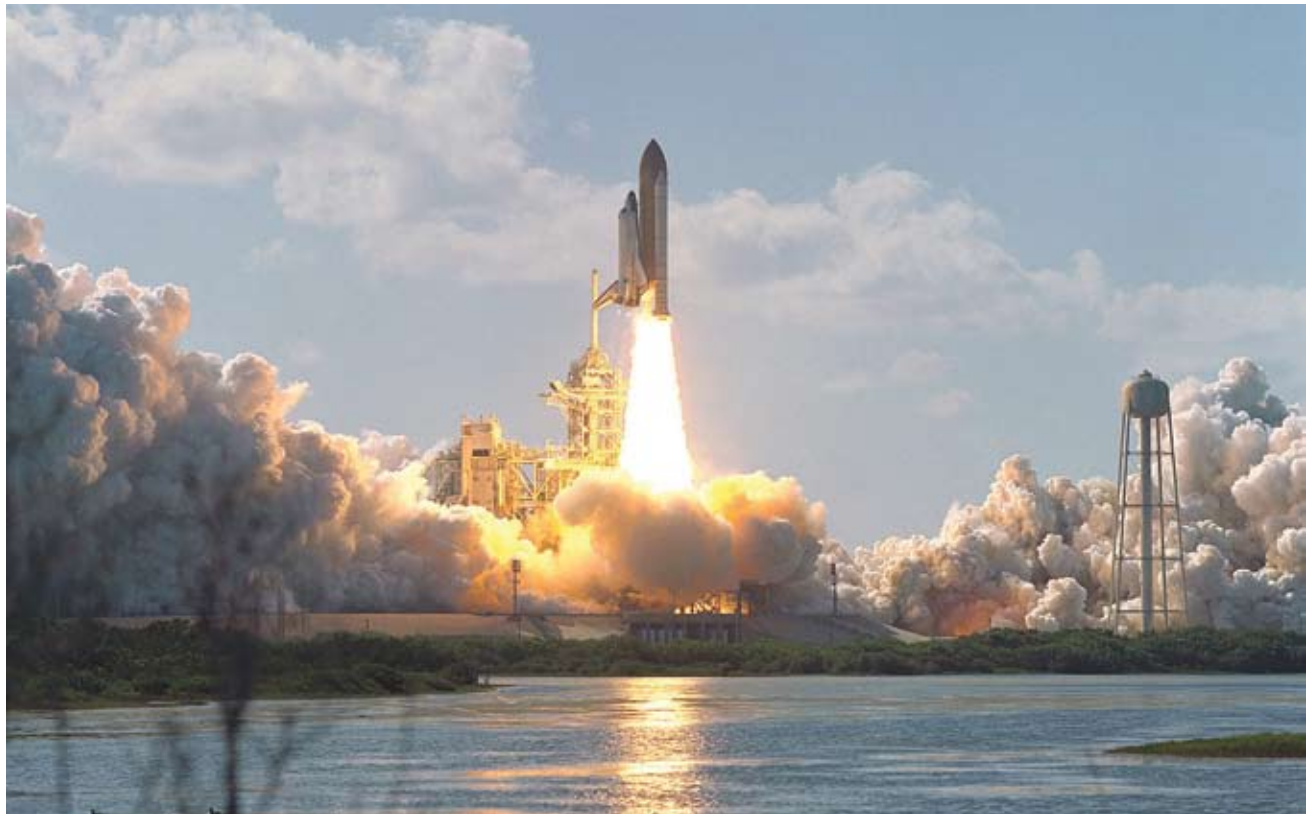
The 290-foot water tank at right of the launch pad holds 300,000 gallons of water that flow through outlets and flame deflectors in the Mobile Launcher Platform just before launch to act as sound suppression. The confluence of the water and intense heat and flames from the three main engines and solid rocket boosters creates the billowing steam seen (flowing left from the main engines and right from the boosters) during this launch of Space Shuttle Atlantis April 8, 2002, on mission STS-110.
